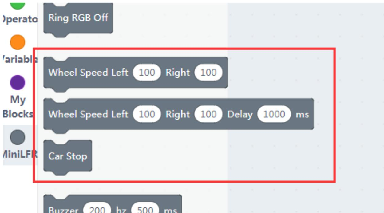
The speed value ranging from -255 to 255. Positive speed makes the motor roll forward, and vice versa. The second block with a delay control, the robot will stop after milliseconds passed.
