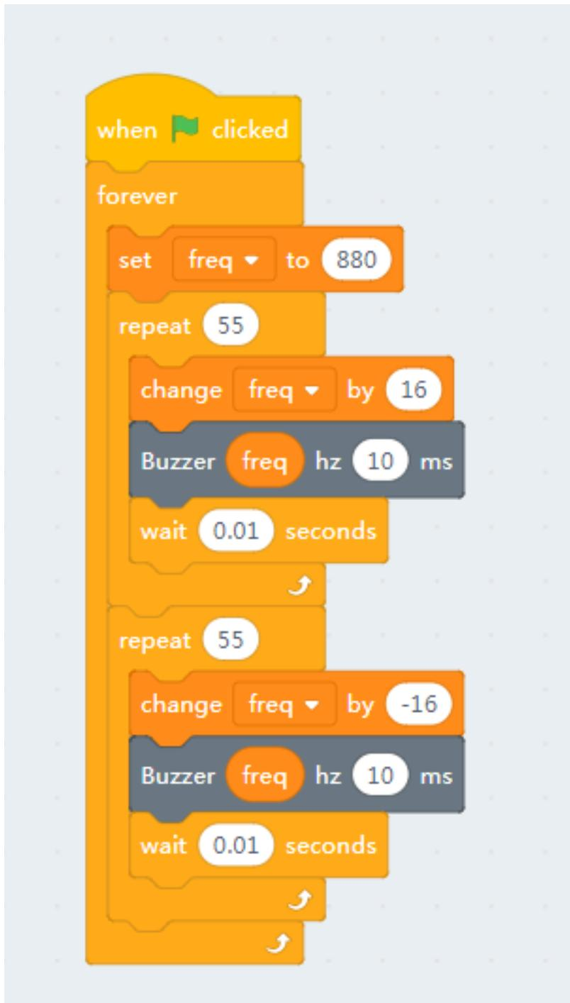
You may find that the effect is a little cracky, no problem, translate it into arduino c++ and burn to the robot and check again. The offline code runs way more smooth than the online mode, this is because in online mode kittenblock send instructions line by line, it takes much time in the communication and instruction decoding.
